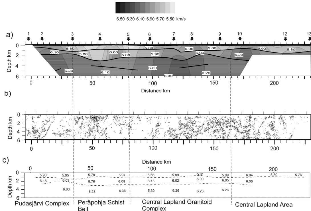
**Figure 1.** The P-wave velocity models. (a) The ray tracing model of the FIRE4. The receiver points are marked with arrows. (b) The FIRE4 reflection profile on the same area as in wide-angle reflection and refraction model (Patisson et al., 2006). (c) The Rayinvr inversion model of FIRE4. The main geological units are marked below the figures and their boundaries are marked with dashed line throughout all models.
