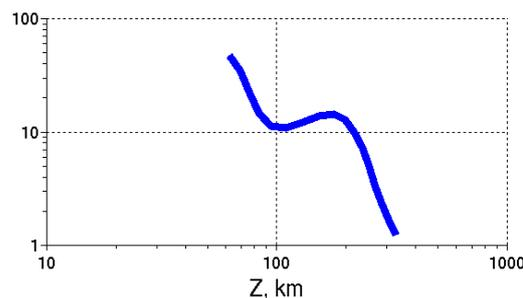
**Figure 3.** Preliminary resistivity model from 1D inversion of HSG response for the site M02. The HSG response is obtained by solving multivariate problem. Note logarithmic depth scale. Note also that shallower structures (crust) are not shown because HSG-analysis has been carried only for periods longer than 1000 s to avoid crustal structures.
