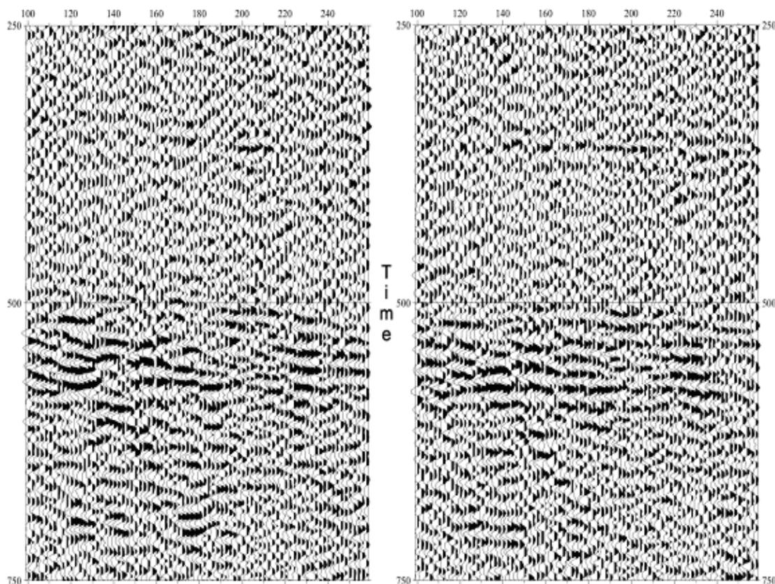
**Figure 3.** Unmigrated stack with refraction static correction (left) and tomographic static corrections applied (right). Refraction static corrections were done by using Hagedoorn's method.
