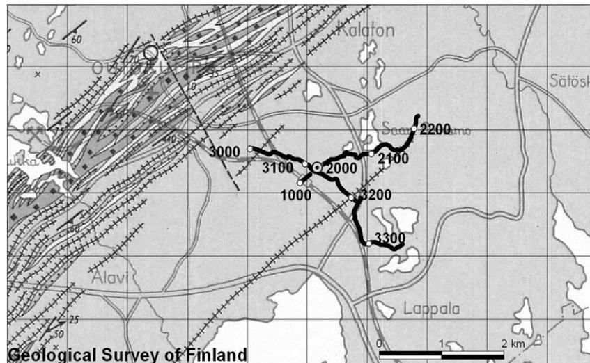
**Figure 1.** Seismic soundings were done on two crooked lines marked in map with numbers. The location of deep drill hole is marked with circle.
