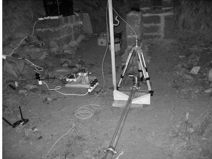
**Figure 1.** Northern end of the NSWT tilt meter in Tytyri mine, Lohja
