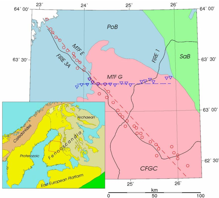
**Figure 1.** Simplified geology of the study area after Koistinen et al. (2001). PoB = Pohjanmaa Belt, SaB = Savo Belt and CFGC = Central Finland Granitoid Complex. Magnetotelluric sites are marked with circles (MTF E) and inverted triangles (MTF G). Dashed lines represent projected profile along which the inversion was carried out. Locations of reflection seismic FIRE 1 and FIRE 3A profiles are shown with lines.
