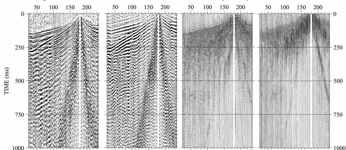
**Figure 2.** Unprocessed field record 2028 and signal response in different frequency bands, 30-40 Hz, 100-150 Hz and 210-220 Hz. Ormsby filter with 10 Hz linear ramps was used to
