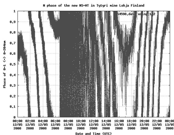
**Figure 2a.** Phase recording of the level sensing interferometer during earthquake 12.5.2008 in China.
