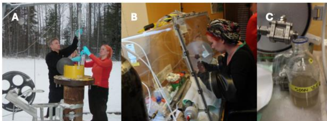
Figure 1. Field sampling in the Outokumpu deep drill hole site. This operation aimed to incubate rock specimens under in-situ conditions at the depths of 500 m and 967 m over a 6-month period. A) Assembling and attaching biofilm traps into the cable. B) Conducting microbiological sampling in an anaerobic field glove box after the experiment. C) Harvesting fluid samples from the closed in-situ biofilm traps.
