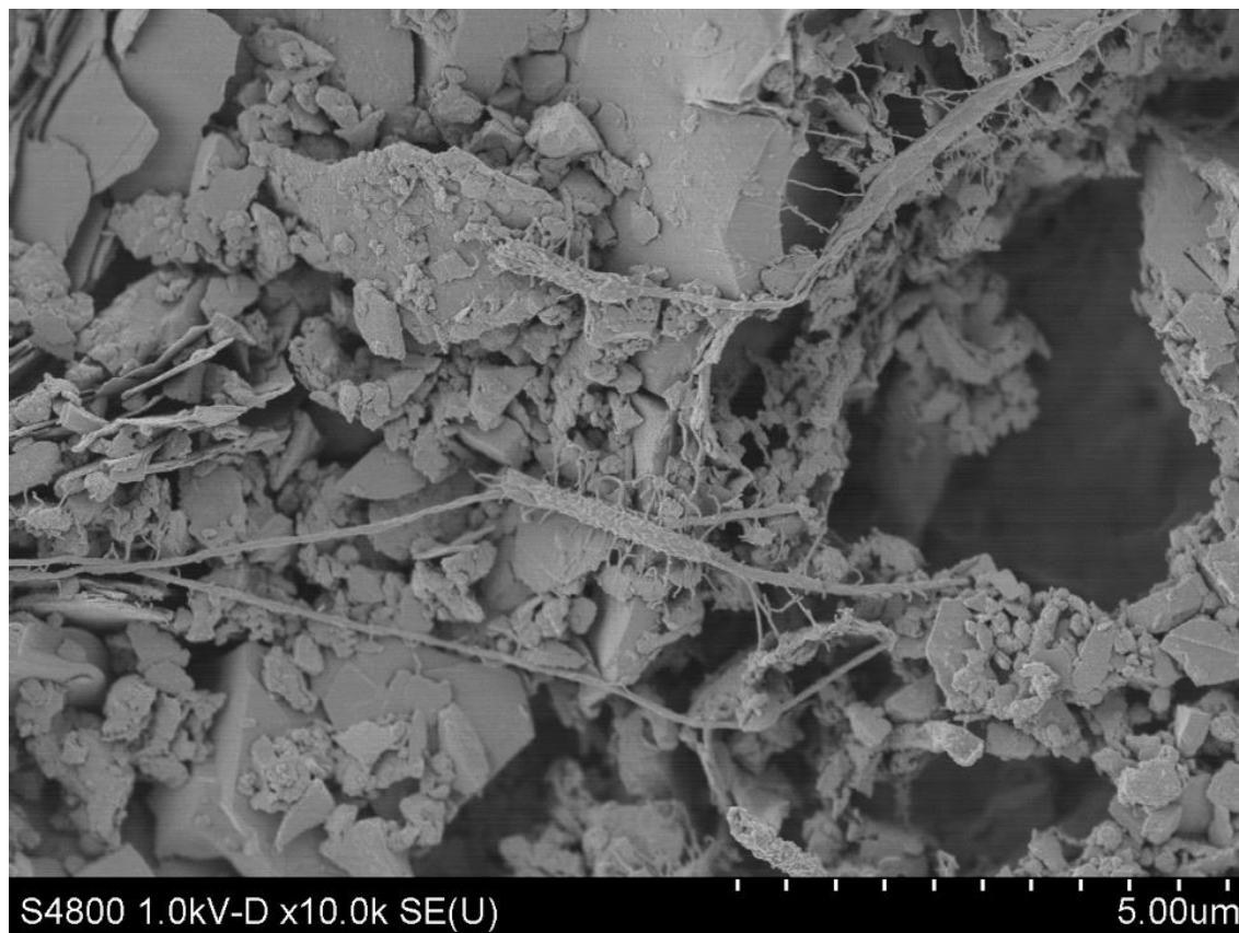
Figure 2. Attached microbial cells on the surface of the mica schist after an 8-month incubation in microcosms with groundwater originating from a depth of 500 m, visualized with SEM. Image by Mari Raulio.
