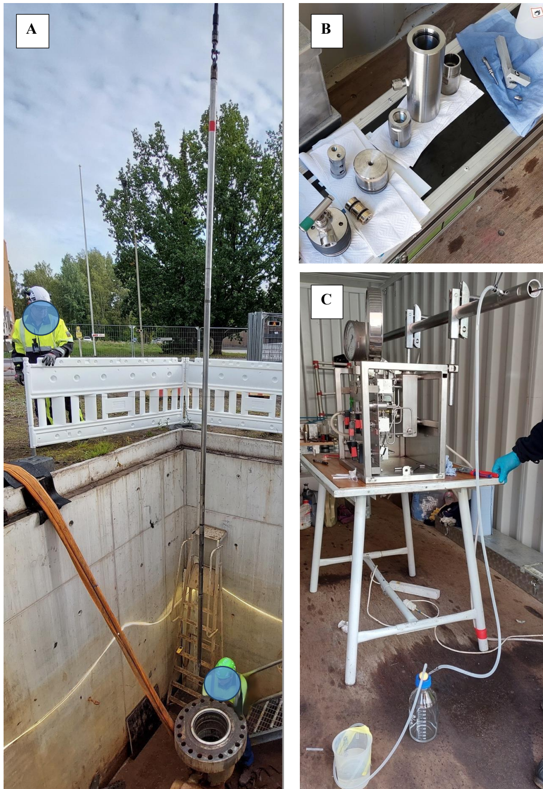
Figure 1. A) Sampler device coming out of the borehole, B) Drying of disinfected sampler parts C) Releasing the sample from the sampler via silicon tube and needle to collection bottle, gas flowing forward to water in a jug.
